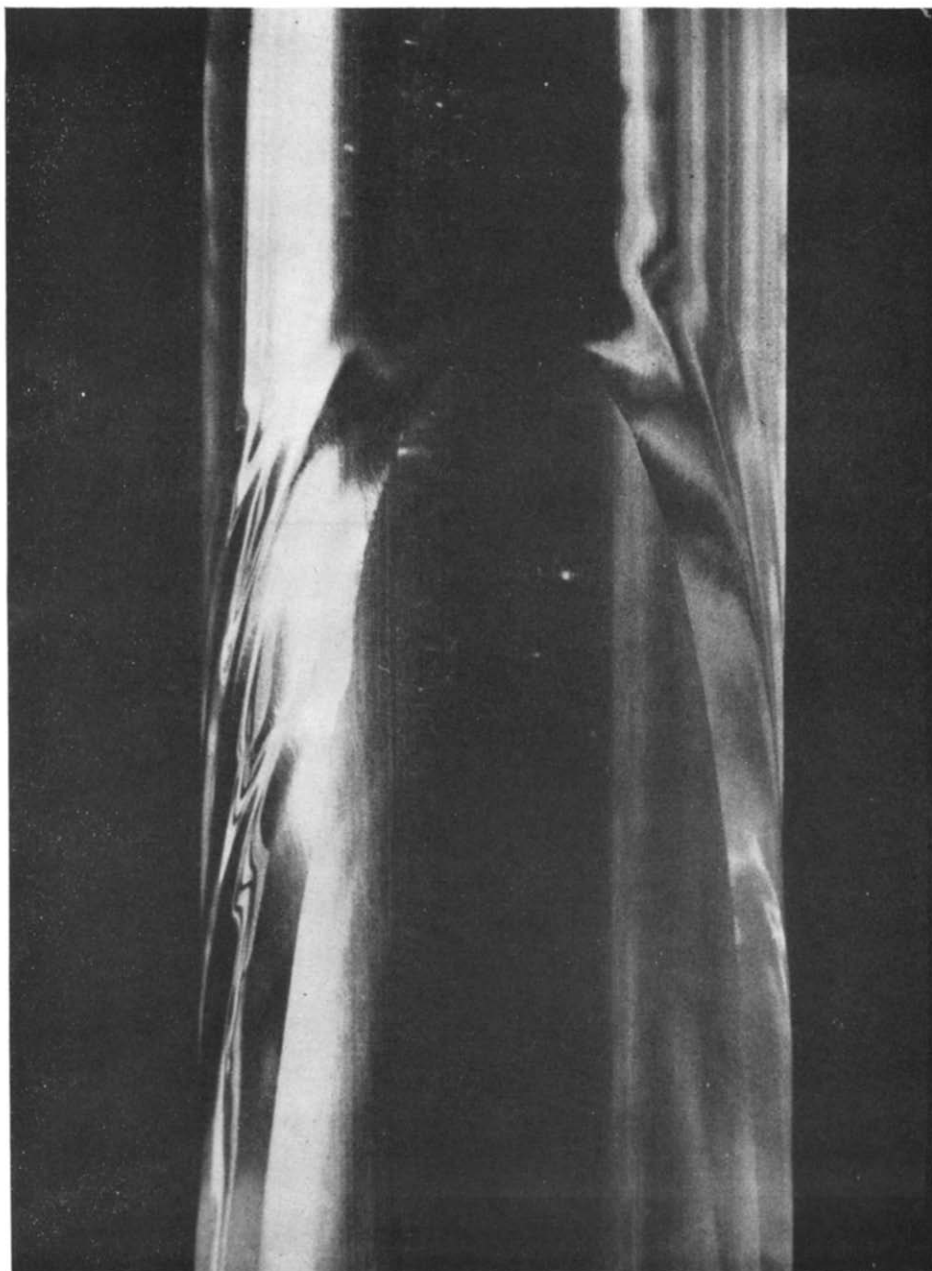
FIG. 4(a). Photograph illustrating film breakdown and formation of a stable patch.
